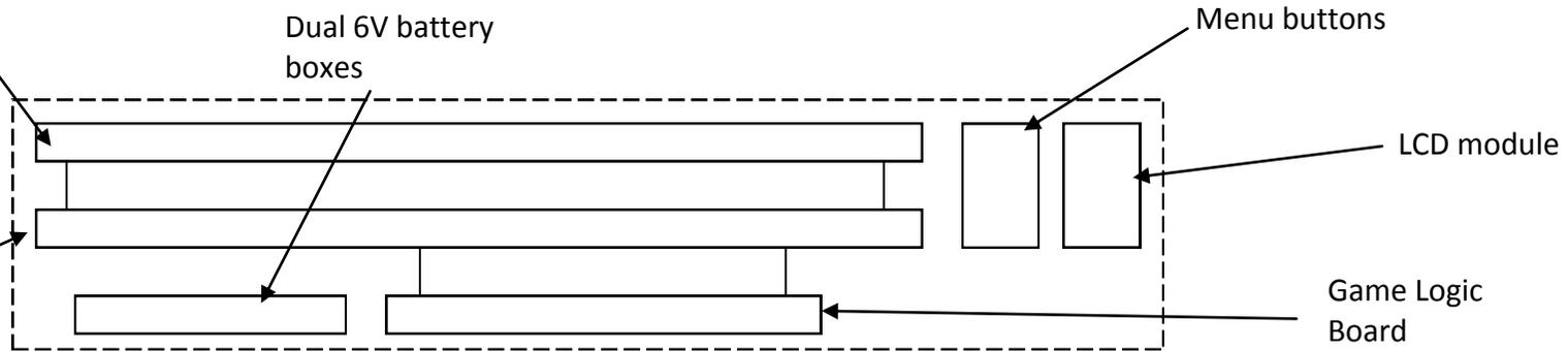
Figure 25.1 - Component Locations Draft - Side View
